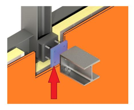
Structural Thermal Breaks can be used in a wide variety of applications where there is a structural requirement of the thermal insulation:
