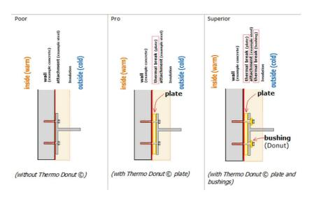
The very tough thermal breaks from "Thermo Donut ©" have a very low thermal conductivity and a very high compressive strength! And even more very important material properties! They are applicable at extreme temperatures (from minus 50 °C (minus 58 °F) up to noncombustible). In addition they have the option "built-in gasket" (pro airtight and contra mold and mildew). The thermal breaks are individually (in almost any size) available.
