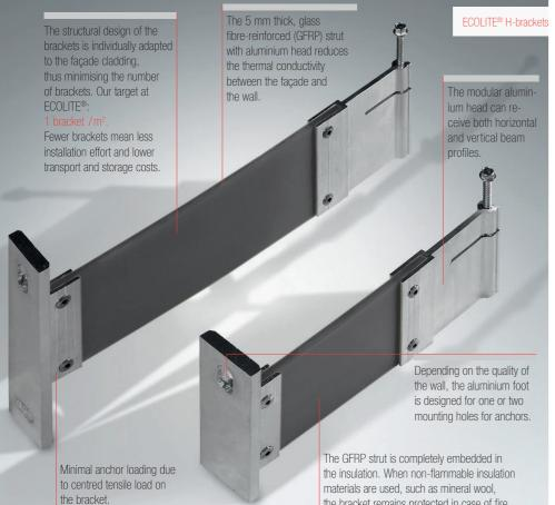
the bracket remains protected in case of fire and its load capacity remains intact.
